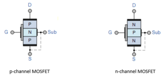
Figure 6: p-channel and n-channel MOSFET [tutorials point].
